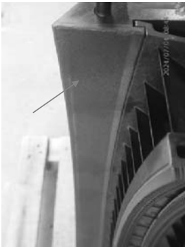
Abradable seal stage 11 as found condition.
