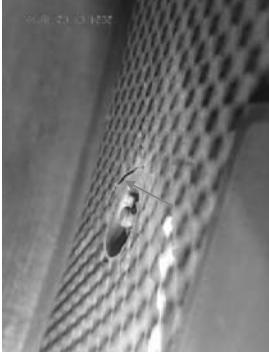
Insulation cassettes damaged at position 5.
