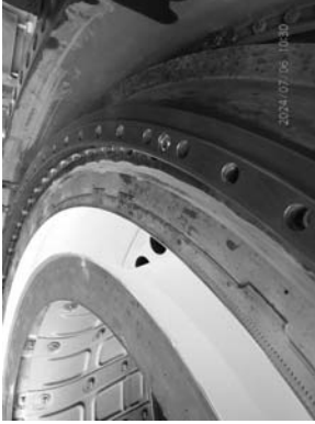
Example of outer outlet ring cooling holes.
