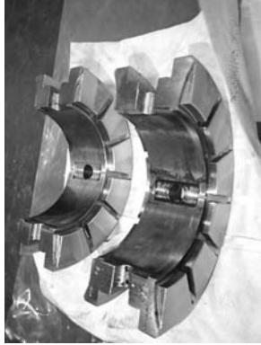
SSS-Clutch bearing 31 overall condition.
