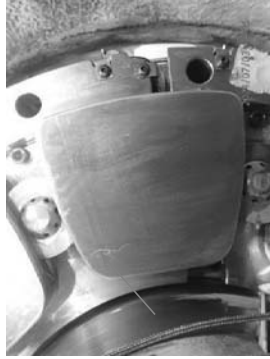
Example axial thrust pad#4 scratched mark.
