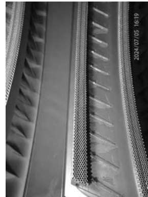
Example of guide vanes stage 5 honeycomb wear condition.
