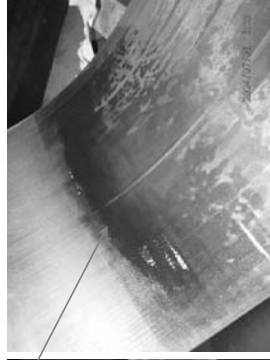
Bearing 11 bottom-half with varnish condition.
