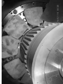
After polishing condition at 0° with PT acceptance. After polishing condition at 45° with PT acceptance.
