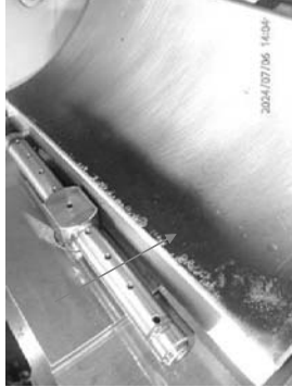
Bearing 22 bottom half cleaned condition.
