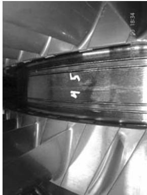
Example of corrosion found between stages 4-5.
