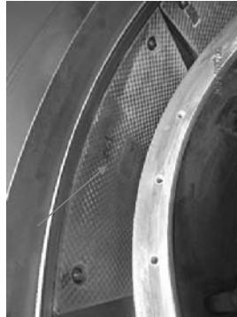
Insulation cassettes at top side not damage.
