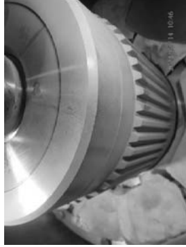
After polishing condition at 180° with PT acceptance. After polishing condition at 225° with PT acceptance.
