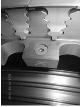
Installed weight on BP5 hole position 11.
