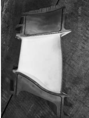
GV2 trailing edge cooling passages overall conditions.
