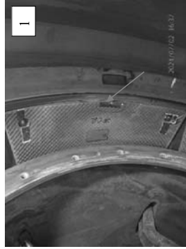
Insulation cassettes damaged at position 1.
