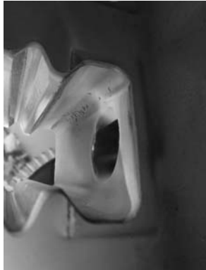
Example view of fir-free condition on Turbine disc#2 and fine dark particles found in the groove.
