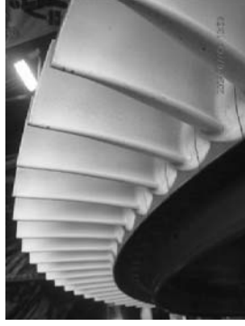
Example blade 2 leading edge overall condition.
