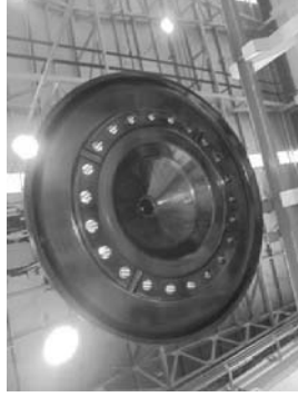
PT applied to rotor hub.
