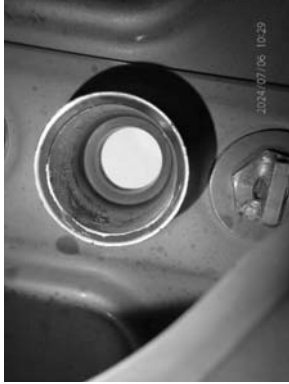
Example of fretting condition at flame detector port.
