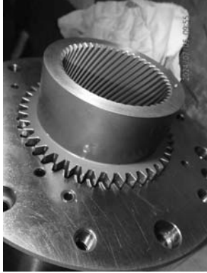
Sliding female splines socket as found condition.
