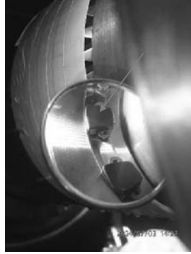
Example closeup reverse thrust pads condition.
