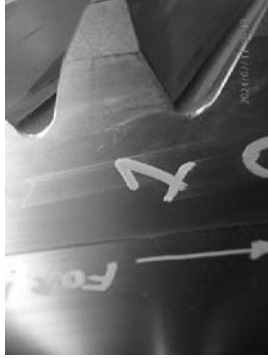
Reference position 1 with macro photos that use to follow up next 10,000 EOH.
