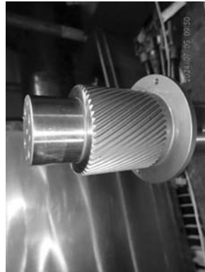
Sliding splines gear overall condition.
