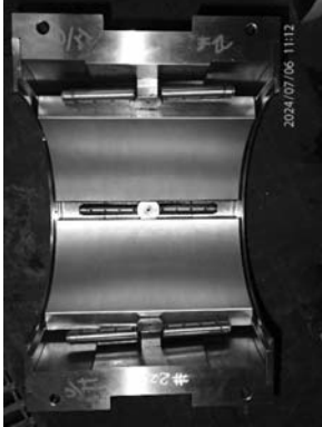
Bearing 22 top half overall condition after cleaned.
