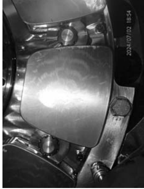
Close view on axial thrust pads before clean.
