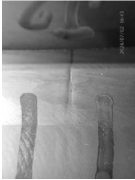
Rear L-profile damaged at position J2.
