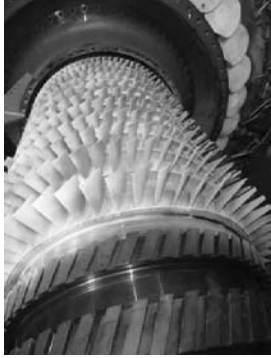
PT were performed on all compressor blades stage 5-15. No relevant indications
