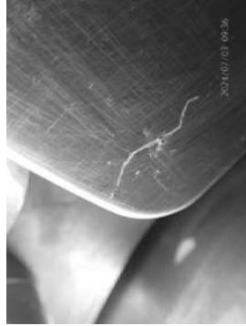
Closeup scratch mark on pad#4.
