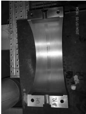
Bearing 12 top half overall condition after cleaned.
