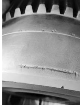
After polishing condition at 90° with PT acceptance. After polishing condition at 135° with PT acceptance.
