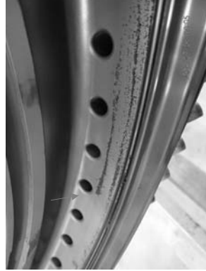
Example of fine dark particles in front of cooling intake to blades "X" side and around the sealing plate "Y" side.
