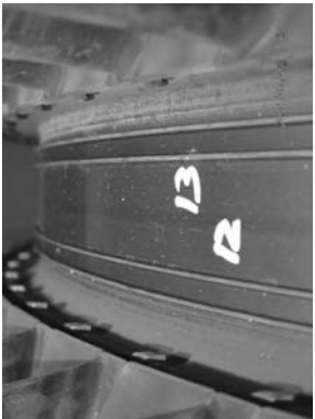
Example of corrosion found between stages 12-13.
