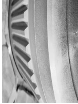
After polishing condition at 315° with PT acceptance.
