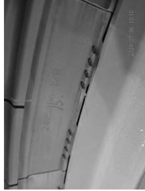
Example of fine dark particles in front of cooling intake to blades "X" side and around the sealing plate "Y" side.
