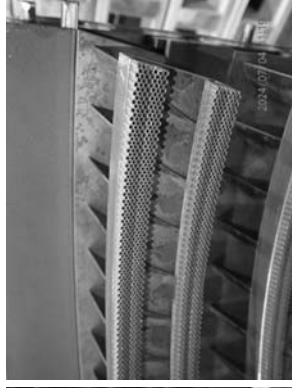
of guide vanes stage 11 honeycomb wear condition
