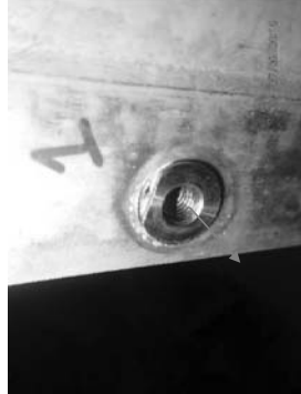
Example threaded insert nuts as found condition not flat with casing.
