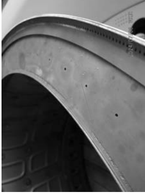
Fretting condition at combustor contact area.
