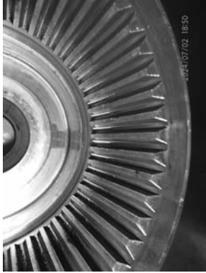
Example closeup on coupling spline condition.
