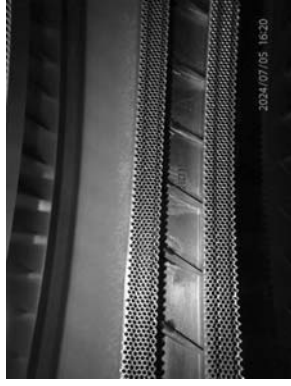
ple of guide vanes stage 6 honeycomb wear condition.
