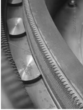
Inner sealing ring honeycomb overall condition.
