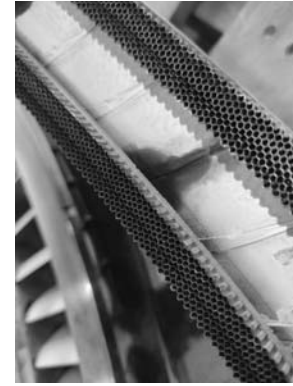
Cracks found by PT on guide vane stage #10 cold side. Cracks found by PT on guide vane stage #15.
