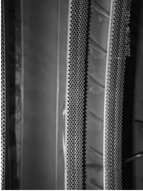
Example of guide vanes stage 13 overall condition. Example of guide vanes stage 13 honeycomb wear condition.
