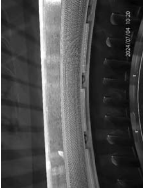
VGV stage 1 inner ring and honeycomb overall condition.
