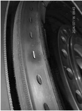
Honeycomb wear condition on swirl generation.
