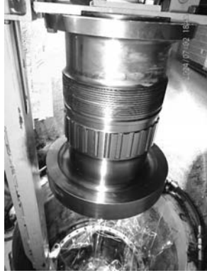
Compressor coupling as found condition.
