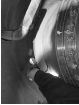
No damage on weld seam behind bearing housing.
