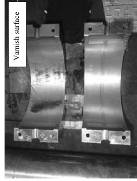
Bearing 12 overall condition before clean.
