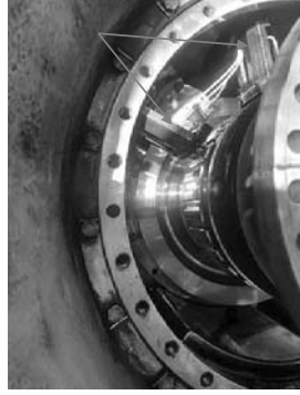
Vibration sensors and speed sensors before dismantled.
