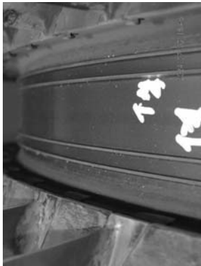
Example of corrosion found between stages 11-12.
