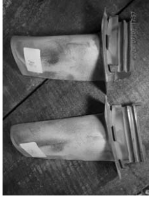
Example of blade 2 suction side overall condition.
