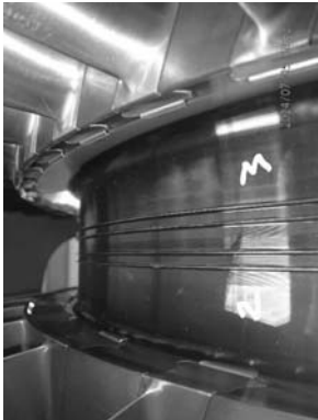
Example of corrosion found between stages 2-3.
