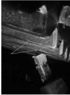
Example FMT photos on suspect wheel cogs area that shown relevant indications (Pitting)
