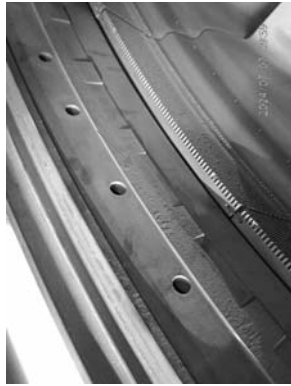
Example of fretting condition against outlet casing.
