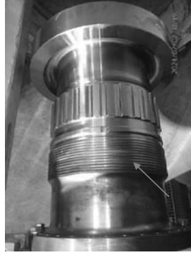
Compressor coupling caulked sealing edge.
