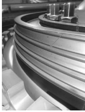
Turned sealing edges inner as found condition.
