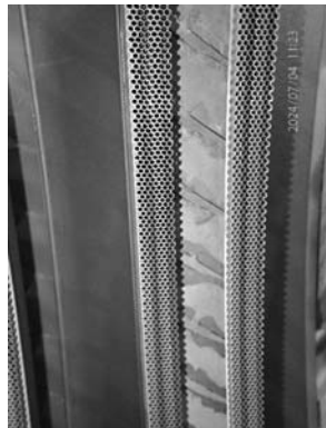
Example of guide vanes stage 14 overall condition. Example of guide vanes stage 14 honeycomb wear condition.
