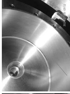
SSS-clutch lube oil chamber cleaned condition.
