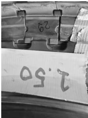
Example view for actual gap at Blade 2 downstream side.
