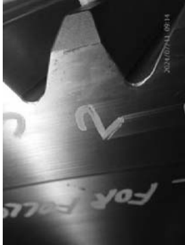
Reference position 2 with macro photos that use to follow up next 10,000 EOH.
