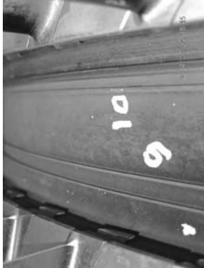
Example of corrosion found between stages 9-10.
