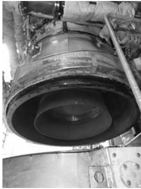
Outlet casing overall condition before dismantling. Observed double nuts missing and loose around fabric bellow.
