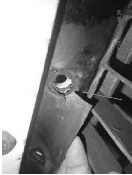
Rubber seal was damaged condition.
