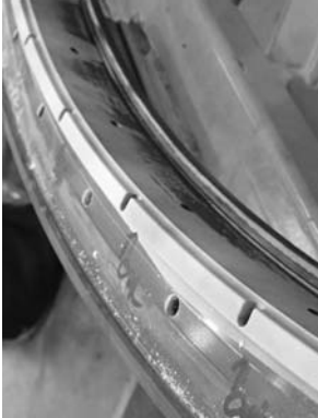
Cracks found by PT in heatshield lugs seating slot
