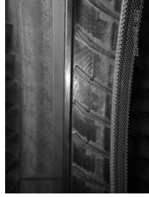
ple of guide vanes stage 8 honeycomb wear condition.
