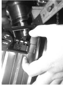
Example corrosion area depth about 0.28 mm.
