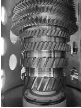
Removed first 4 stages blade to upgrade to B3 package.
