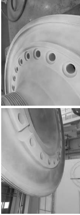
PT on rotor hub by water washable method, no relevant indication.
