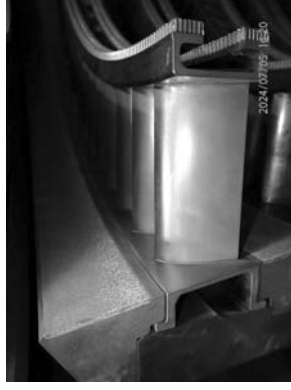
Example of guide vanes stage 6 overall condition.
