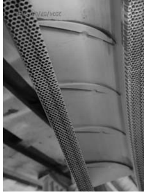
Cracks found by PT on guide vane stage #3 cold side. Cracks found by PT on guide vane stage #10.
