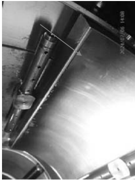
Bearing 21 top half varnish condition.
