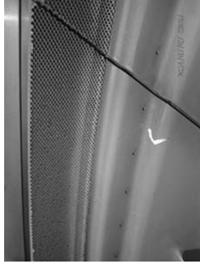
Minor contact marks found on GV3 extruded casing area.
