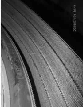
Outer sealing ring honeycomb overall condition.
