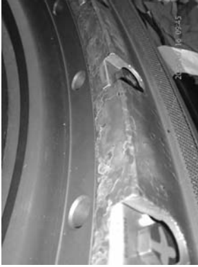
Honeycomb wear condition on swirl generation.
