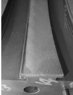
Example of abradable seal stage 14 overall condition.
