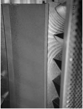
Condition of abrasible seal stage 9.
