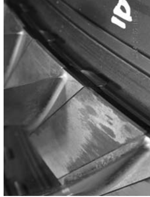
Example of compressor rotor stage 10 condition.
