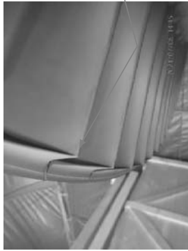
Example of blades 3 minor rubbing at leading edge.
