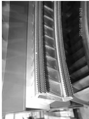
Example of guide vanes stage 4 honeycomb wear condition.
