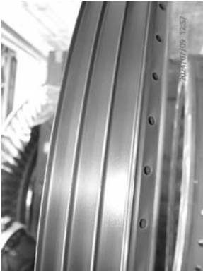
Close up on sealing ring 2-3 seating slot.
