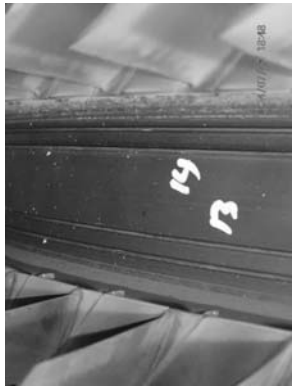
Example of corrosion found between stages 13-14.
