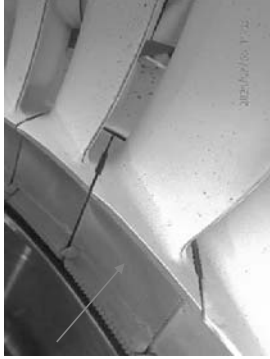
No axial contact mark on G12.
