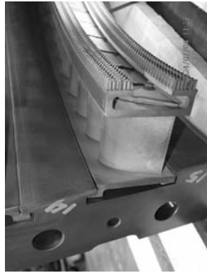
Example of guide vanes stage 14 overall condition. Example of guide vanes stage 14 honeycomb wear condition.
