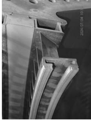
Condition of abrasible seal stage 10.
