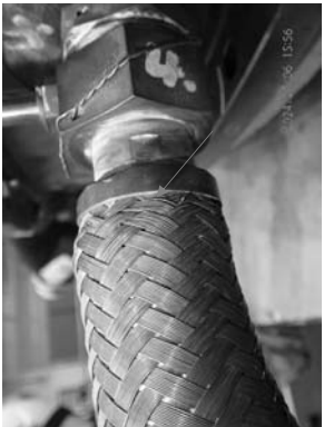
Example view on GV2 cooling hose, flexible thread damaged (left) and hose deformation (right).
