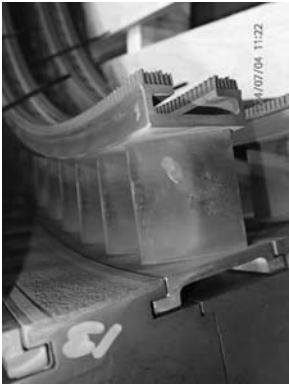
Example of guide vanes stage 13 overall condition. Example of guide vanes stage 13 honeycomb wear condition.
