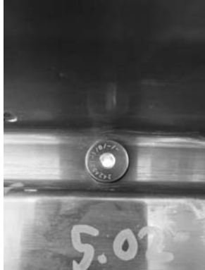
Heat shield cooling air supply plug after modified by add 45 deg chamfer.
