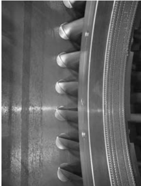
VGV stage 2 inner ring and honeycomb overall condition.
