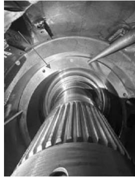
Installed new shim 1.55 mm in place behind bearing#1.
