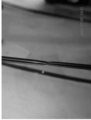
Example of deformed condition found on split e-sealing.
