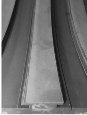
Example of abradable seal stage 13 overall condition.
