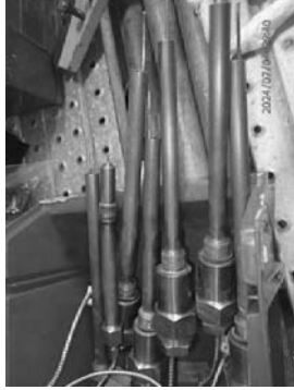
C1 probe end thread as found condition.
