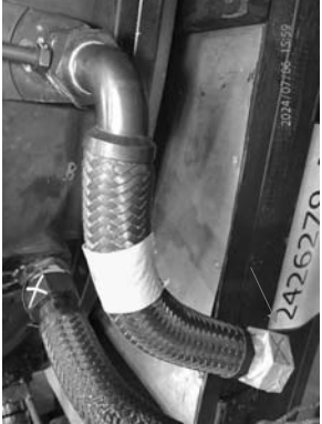
Example view on GV2 cooling hose, flexible thread damaged (left) and hose deformation (right).
