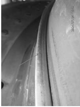
Front L-profile wear mark around circumference.
