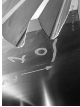
Reference position 0 with macro photos that use to follow up next 10,000 EOH.
