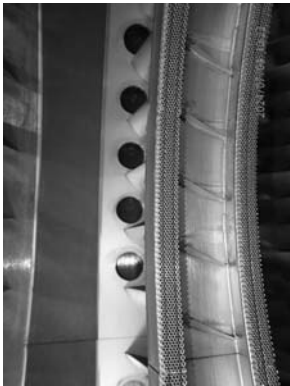
Example of guide vanes stage 3 honeycomb wear condition.
