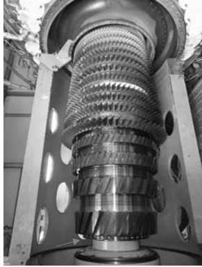
Balancing weight location on BP2.
