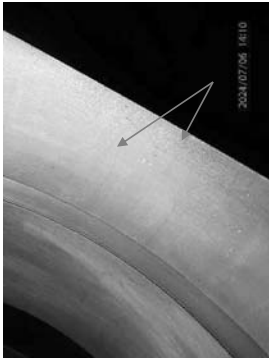
Bearing 12 bottom half found unsmooth surface.
