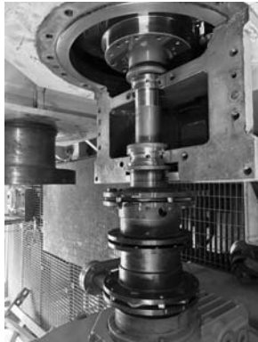
SSS-Clutch connected with flexible coupling overall condition. SSS-Clutch overall condition.
