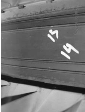
Example of corrosion found between stages 14-15.
