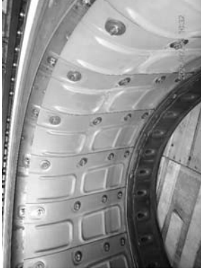
Inner heatshield seen from turbine side overall condition. Combustion diaphragm and turbine flange disassembly.
