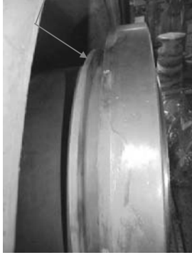
Applied PT on compressor rotor nuts area that found lacking mark from removal turbine module process.
