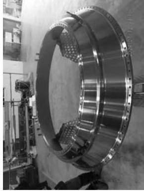
New combustor during performed the measurement.
