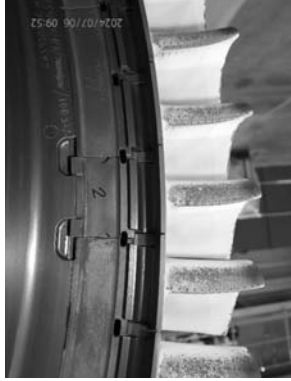
Actual gap at Blade 1 position 2 upstream side.
