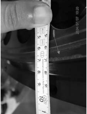
Pretting condition from contact with combustor.
