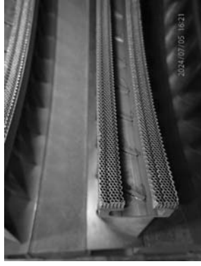
ple of guide vanes stage 7 honeycomb wear condition.
