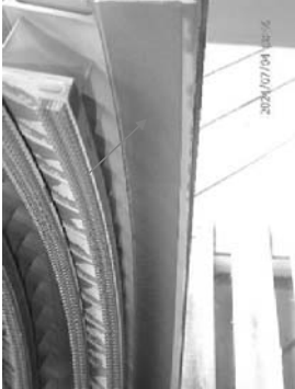
Abradable seal stage 15 as found condition.
