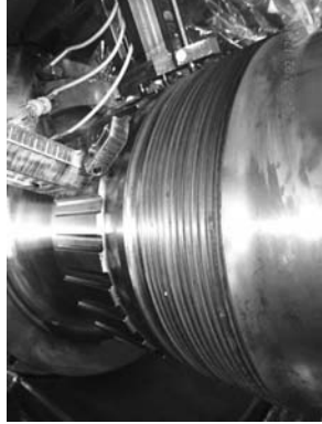
Compressor coupling caulked sealing edges condition.
