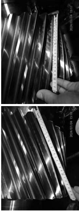
Example of white mark on pinton cogs starter motor side (left) and turbine side(right).
