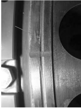
Main inner ring fretting mark were close to limit of serviceable condition.
