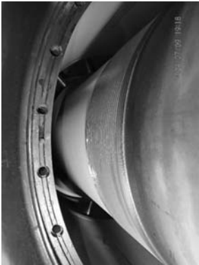
Compressor rotor turned seals at bottom location.
