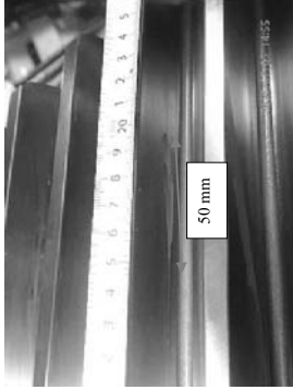
Ref#4 electro discharge on wheel cogs (Gen side)
