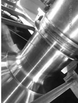
Low speed journal area on wheel shaft as found condition.
