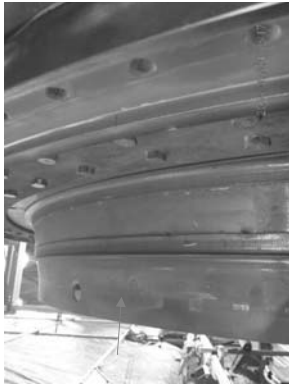
Example of fretting found at front lip area.
