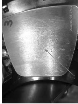
Axial thrust pads#3 over-heated area.
