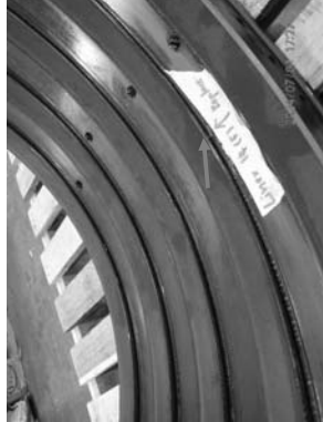
Spacer ring front liner stage 14 found damaged.
