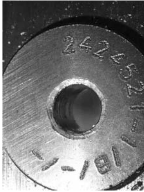
Heatshield I cooling hole overall condition.
