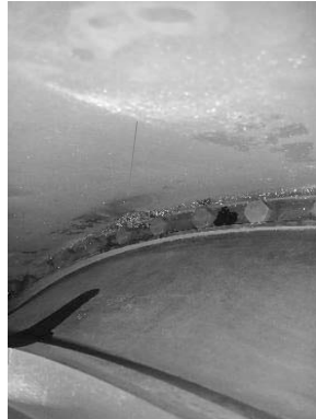
Debris deposit around Turbine flange.
