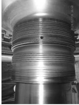
Caulked sealing edges overall condition.
