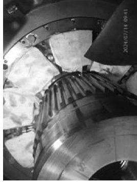
Example damaged spigot surface 1&2 at 31.5° position. PT was performed after polishing finish to confirm defect.
