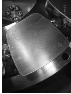
Example axial thrust pad #7 scratch mark.
