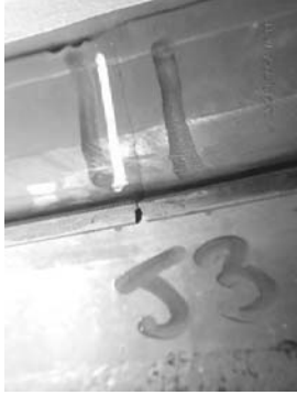
Rear L-profile damaged at position J3.
