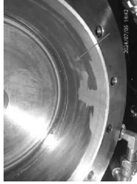
SSS-clutch lube oil chamber varnish condition.
