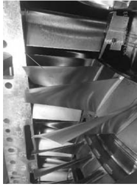
Compressor blades stage 2 as found conditions.
