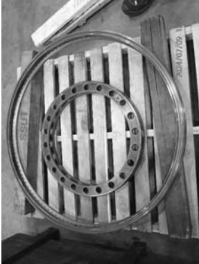
Sealing ring (Old) between disc 2-3 overall condition.
