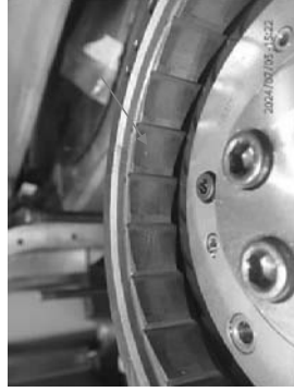
Ratchet side teeth cleaned condition.
