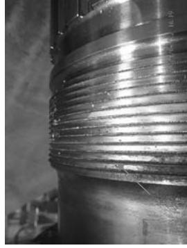
Caulked seal edge cleaned condition.
