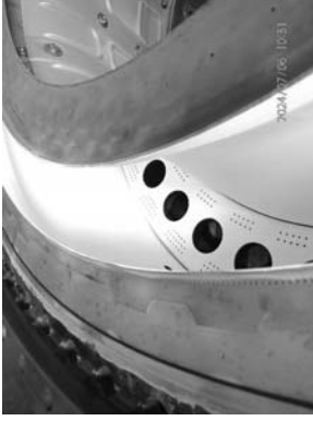
Example of inner outlet ring cooling holes.
