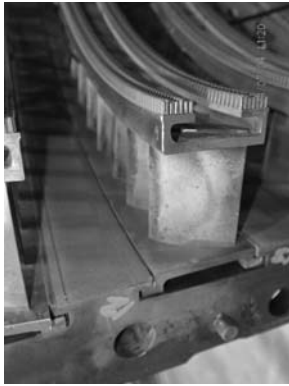
Example of guide vanes stage 12 overall condition. Example of guide vanes stage 12 honeycomb wear condition.
