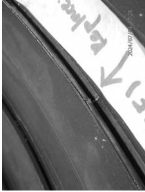
Close up view around damaged point on spacer ring front liner stage 14.
