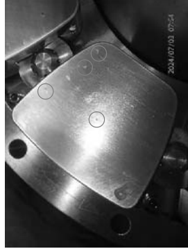
Example axial thrust pad #9 pitting damaged.
