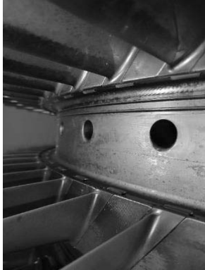
Example of corrosion found between stages 8-9.
