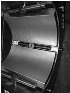
Closeup condition on the top pad of bearing 22 top half.
