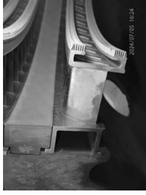
Example of guide vanes stage 10 overall condition.
