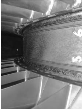
Example of corrosion found between stages 5-6.
