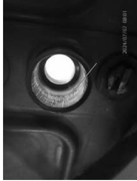
As condition flame detector hole was fretting.
