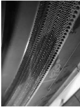
Main inner ring honeycomb as found wear condition.
