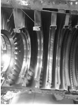
GV link arm control dismantling and shim replaced.
