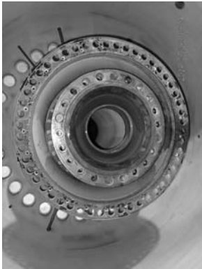
Compressor rotor spigot fit area overall condition.
