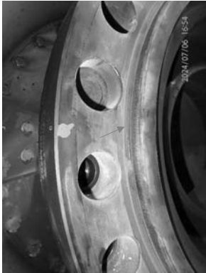
Example close view on spigot fit surface condition.
