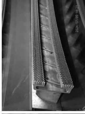
2 of guide vanes stage 9 honeycomb wear condition.
