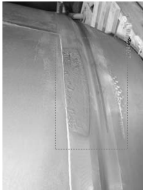
Example view for contact marks on outlet cone (Big wok).
