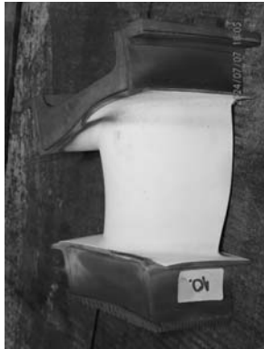
Oxidation noticed on leading edge inner platform of GV42.
