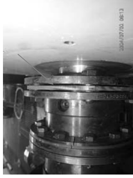
Shim pack at gearbox side condition.
