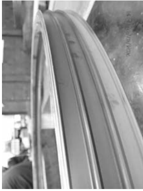
Close up on sealing ring 1-2 seating slot.
