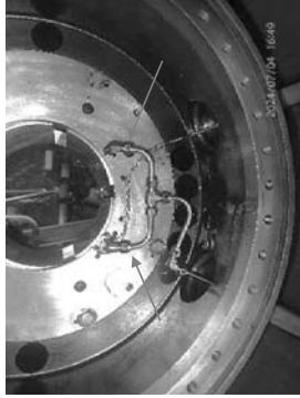
Jacking oil tubing that connect to bottom pads.
