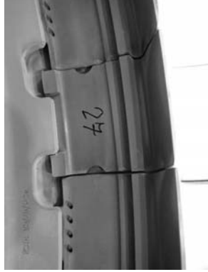
Example view for actual gap at Blade 1 position 27 (left) and 52 (right) for downstream side.
