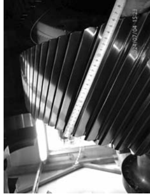
Example of white mark on wheel cogs generator side (left) and turbine side (right).
