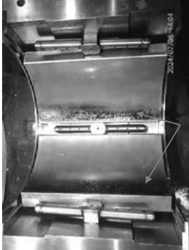
Bearing 22 top half overall condition before clean.
