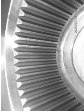
Closeup spline cleaned condition.
