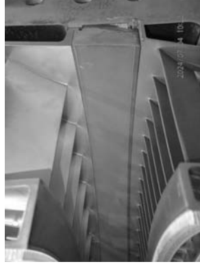
Condition of abrasible seal stage 4.
