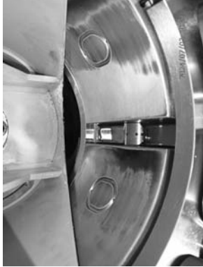
Example of as found condition on radial jacking oil pads.
