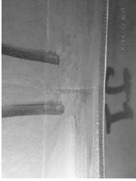
Rear L-profile damaged at position J1.
