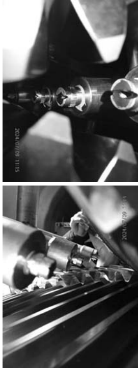
Example view on tip nozzle oil sprays after direction adjustment (left-top manifold and right-bottom manifold).
