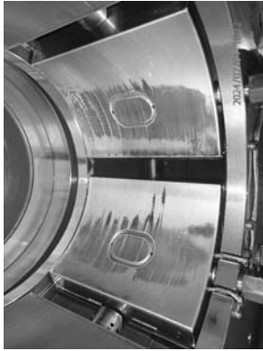
Jacking oil pad before clean condition.
