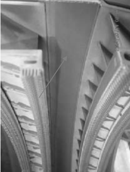
Abradable seal stage 14 as found condition.
