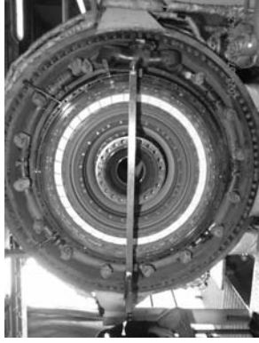
C&D measurement on GV1 stator and rotor.
