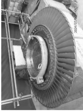
Example of downstream blade stage 3.
