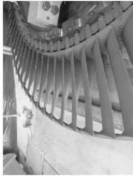
Example of turbine blades 3 trailing edge side.
