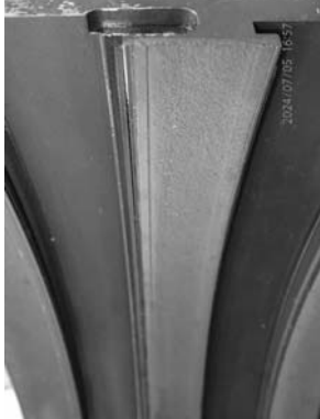
Example of abradable seal stage 12 overall condition.
