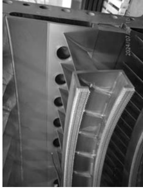
Condition of abrasible seal stage 3.
