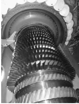
PT were performed on all compressor blades stage 5-15. No relevant indications
