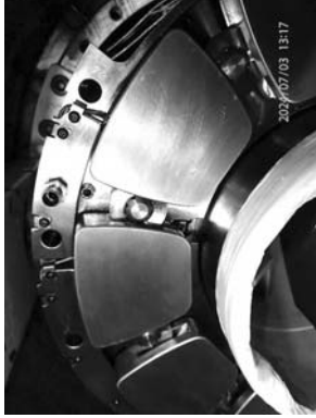
Example of axial pad after cleaned condition.
