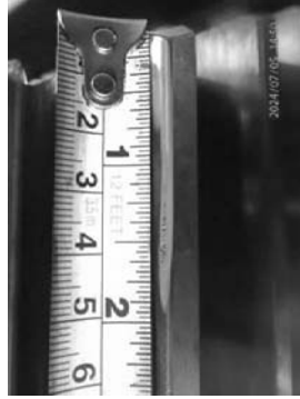
Example corrosion area length about 19 mm.
