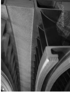
Condition of abrasible seal stage 7.
