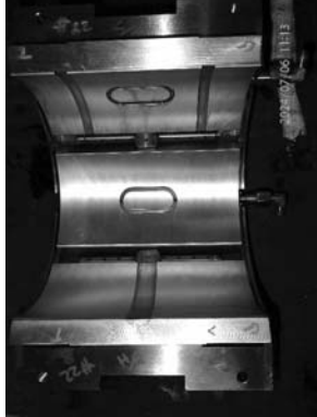
Bearing 22 bottom half overall condition after cleaned.
