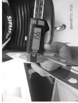
New spacer shim thickness is 1.55 mm.
