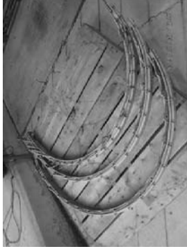
GV link arms dismantled and LYDT was installed.
