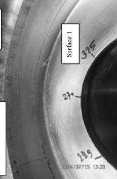
After polishing spigot surface 1&2 at 270° position.
