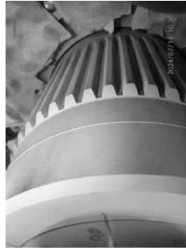
After polishing condition at 90° with PT acceptance. After polishing condition at 135° with PT acceptance.
