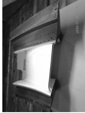
Mild oxidation conditions on CV1 suction side (left) and leading side (right).
