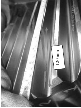
Ref#2 electro discharge on wheel cogs (Gen side)
