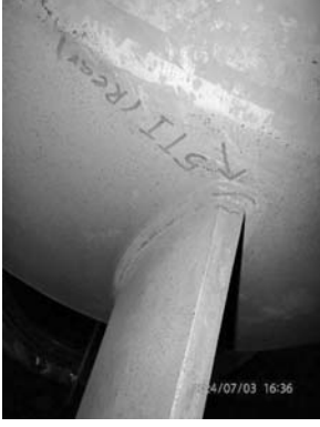
Example view for cracks on weld seam of rear support struts.
