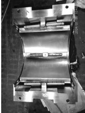
Bearing 22 top half overall condition before clean.
