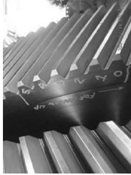
Reference location 6 positions at wheel cog are same erosion and electro discharge.
