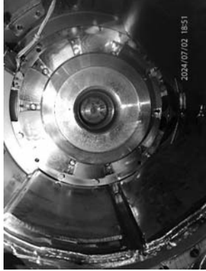
Axial thrust pads as found overall condition.
