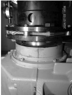
Shim pack at starter motor side condition.
