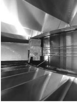
Turned seal condition between stage 2 and 3.
