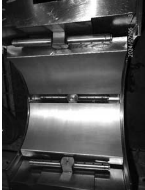
Example of closeup condition on the top pad of bearing 21.
