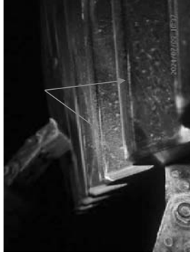
Example FMT photos on suspect wheel cogs area that shown relevant indications (Pitting)
