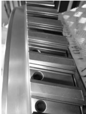
Example view of fir-free condition on Turbine disc#2 and fine dark particles found in the groove.
