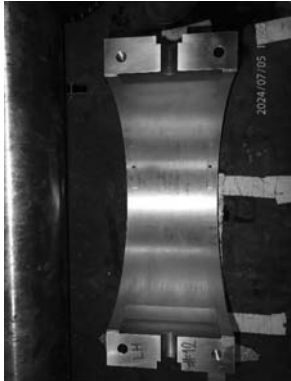
Bearing 12 bottom half overall condition after cleaned.
